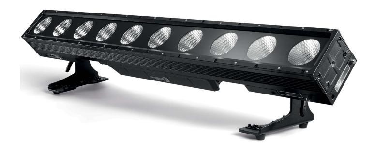
The CLF LEDbar PRO is a multifunctional linear LED batten. Because of the 24° beam angle it can be used as cyclorama as well as pixel controlled effect machine. 10 Big, individually controllable, high power RGBW LEDs deliver a rich color set and smooth HD dimming. Dynamic effects are easily configured by DMX, but the CLF LEDbar PRO is also Art-Net and sACN ready.
